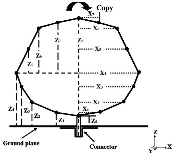
Fig.1 Structure of Planar monopole antenna
