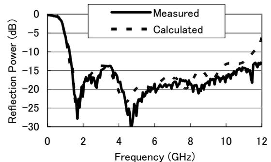
Fig. 6 Comparison of measured results to calculated results of antenna (b)
