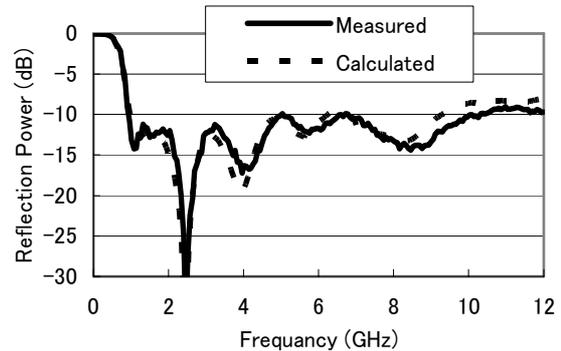
Fig. 5 Comparison of measured results to calculated results of antenna (a)
