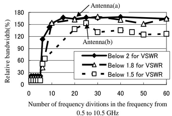
Fig.3 Relationship between number of frequency divisions in the frequency band and relative bandwidth
